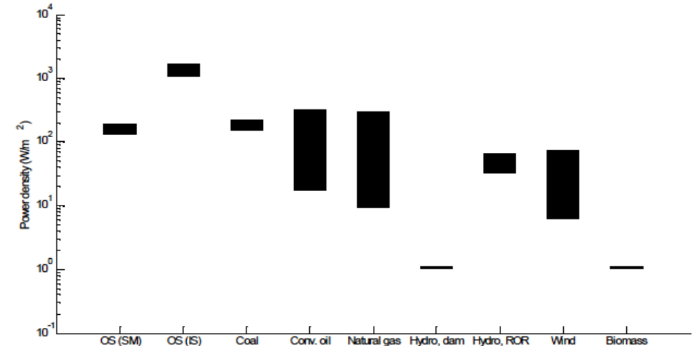
Figure 1. Power densities (W/m 2 ) of energy production in Alberta. OS, IS and OS, SM are in situ oil sands and surface mining of oil sands. ROR is run of the river hydropower (Jordaan, 2010).
